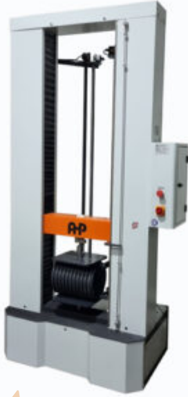
Ring Stiffness Tester According to ISO 9969-50KN-2000mm DevamÄ±nÄ± oku
