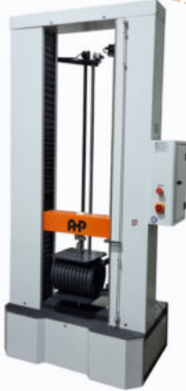
Ring Stiffness Tester According to ISO 9969-100KN-630mm DevamÄ±nÄ± oku
