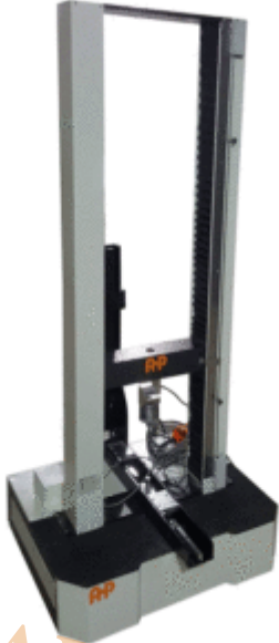
Welding Strength Tester for UPVC Profiles-20KN DevamÄ±nÄ± oku
