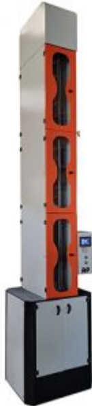
Falling Weight Impact Tester-OD:400-H:2000mm Read more
