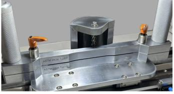
TEMPCUT is a laboratory machine offered from AHP PLASTIK MAKINA to cut and mill hard plastic materials into standard dumbbell shape specimens for tensile test such as ASTM D638 and more.
