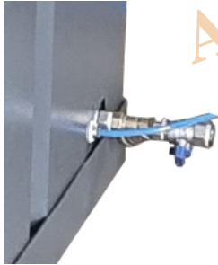
6mm compressed air line input
