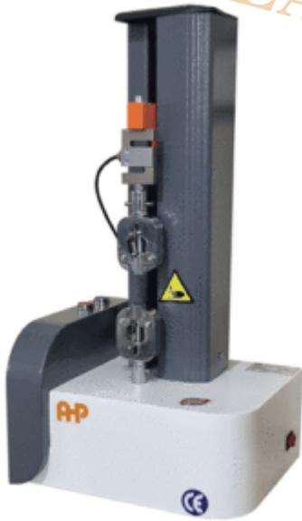
[Single Column Tensile Compression Tester \(UTM\)](#)
