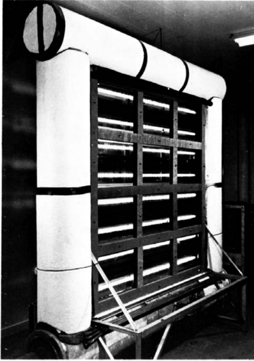
FIG. 1 Typical Accelerated Weather Cycle Test Apparatus
