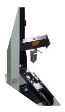
Welding test fixture for UPVC Profile
