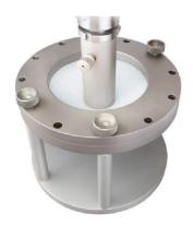
Static Puncture Test (CBR test) according to ISO 12236
