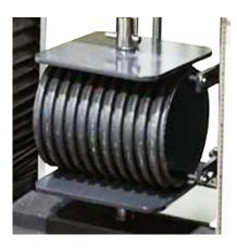
Ring stiffness Test fixture 300x300mm
