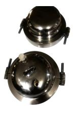
End Caps for Hydrostatic Pressure Testing
