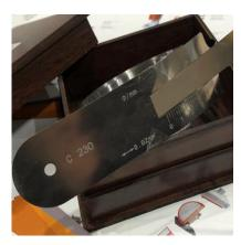
Circometer PI Tape – Diameter Measurement Tape
