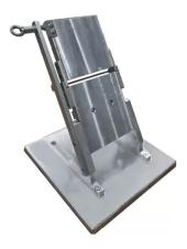
Bending Test Apparatus - ISO 4675
