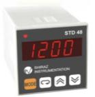
1- Hold "Mode" and "down arrow" key simultaneously for 5 seconds until "tyP" is indicated on the screen. Then release the keys. KMAKINA
