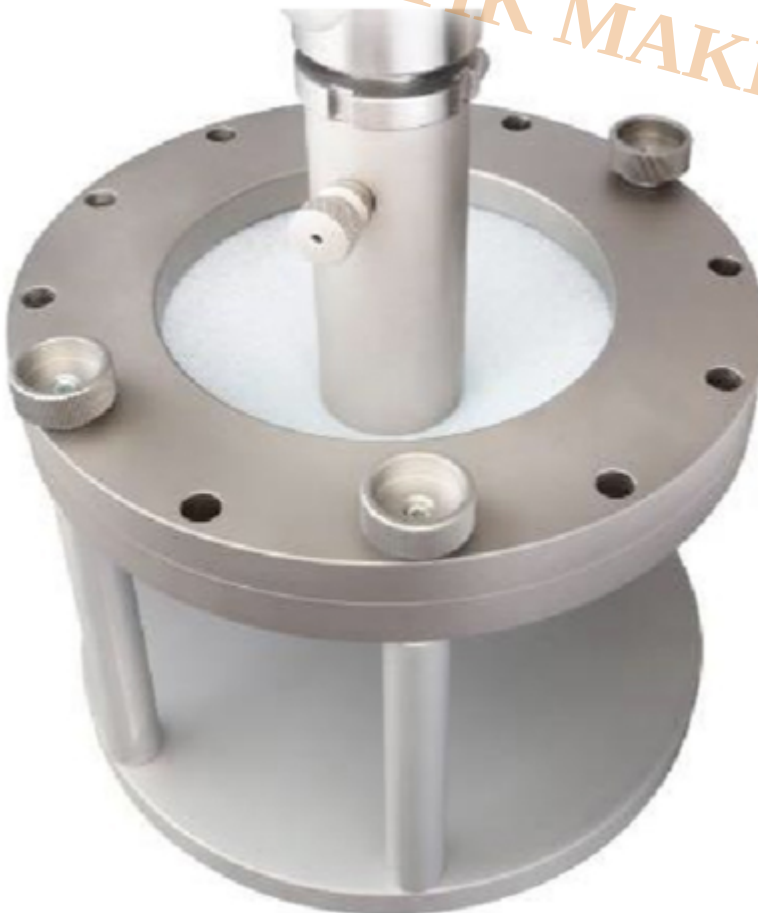
Figure 2. AHP static CBR puncture fixture. The ring clamp secures the specimen while the plunger applies the puncture load. View product.
