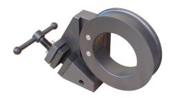
This manual capstan grips are used for testing high capacity ropes. The test specimen is wrapped one or more times around the capstan before being clamped with jaws. The capstan roller generates a slow notch free stress relief to prevent the breakage of the specimen in the jaw clamping area. The number of wraps depends on the sample's coefficient of friction.
