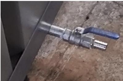
12- Connect drain hose. It is paced in the back top side of the bath
