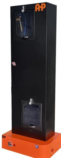
**Cabin for Wet Retroreflection Measurement According to ISO 20471**
