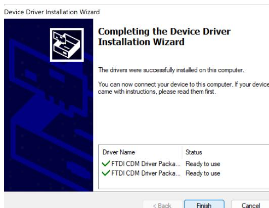
7- After installation, refer to (Device Manager/Ports) from control panel of Windows and check if you have virtual COM port
