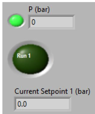
When the connection of PC to the machine is correct the led will be green and current pressure value will be displayed on "P (bar)". When you click start button the "Run1" indicator will be green. "Current setpoint 1 (bar)" will be changed as per setting value for pressure increase rate.
