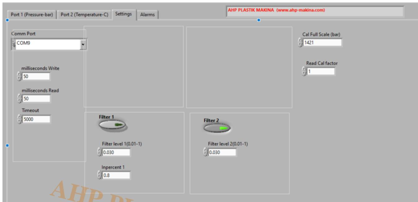
When you set a definite pressure for the sample and pressure dropped suddenly by (1-inpercent) the pressure line will be stopped automatically. Suppose you set pressure to 800 bar and  $\text{inpercent}$  value is 0.8 for sample piece. This means, if the pressure dropped suddenly by  $(1-0.8) \times 800 = 160$  bar line will be stopped. This is important parameter for recognizing the sample burst.
