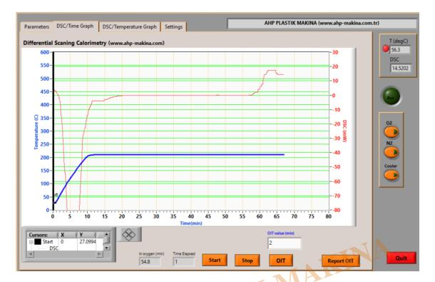
After setting the parameters in the first page now you can start the test. Click on "Start". When you click start you will hear sound of solenoid valve for N2 gas. It will be opened automatically after clicking on Start. When the temperature reaches set value, a timer will be start counting. This is the timer that after passing this time N2 gas will be switched automatically to O2 gas. This time can be set in setting page with the name of "Delay(Sec)".
