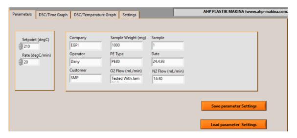
For OIT measurement you need to set two main parameters of "Setpoint(degC)" and "Rate(degC/min)".
