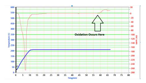
After oxidation occurs "Stop" the test and drag the "End" cursor to the break point. This process can be automatically done when you export data to "Advantage" software. After you dragged end cursor to break point click on "OIT" key and oxidation time will be calculated.
