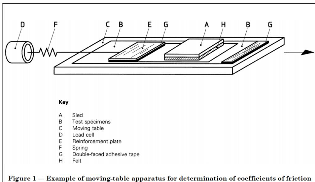
**5.2** The test device shall comply with the following conditions.
