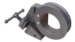
This manual capstan grips are used for testing high capacity ropes. The test specimen is wrapped one or more times around the capstan before being clamped with jaws. The capstan roller generates a slow notch free stress relief to prevent the breakage of the specimen in the jaw clamping area. The number of wraps depends on the sample's coefficient of friction.
