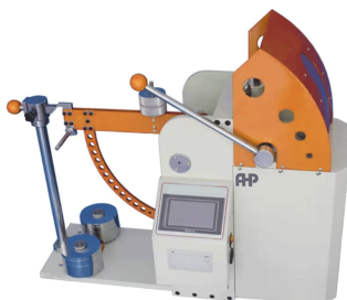
CardBoard Puncture Tester According to DIN 53142-1
