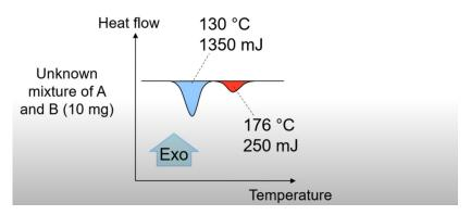
Here is the DSC graph of the mixture. The total weight is 10 mg of the sample piece. Total energy for each peak is measured, 1350 mJ and 250 mJ. Specific enthalpy is calculated based on the total energy divided by mass of the sample.
