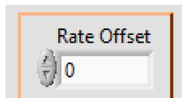
In the above example calculated rate is 23.3C/min While we set to 20C/min. then need to set rate offset value as -3.3C/min.
