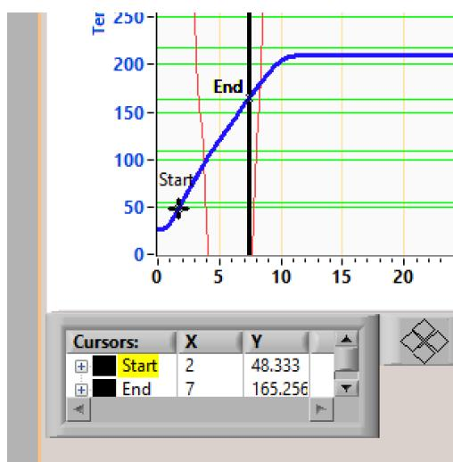
In the bottom section of graph you see data for two cursors. time and temperature data for that two cursor is indicated. you can easily calculate the slope of the line.
