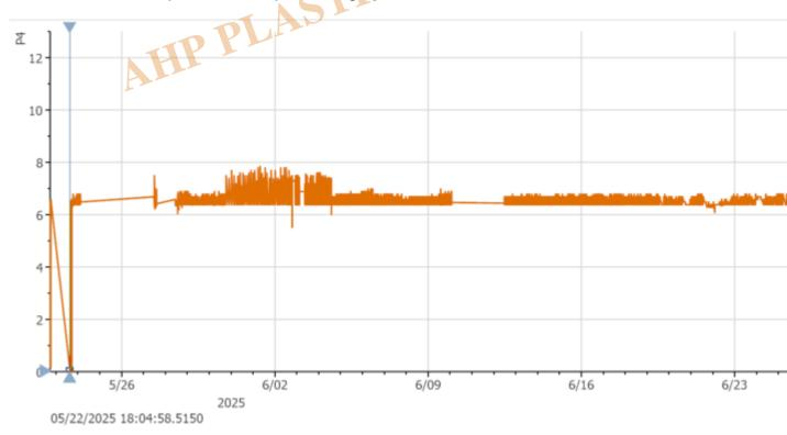
Line No.4 had some out-of-range pressure in some time periods. When a line pressure shows fluctuation during a test, it means that there is absolutely tiny leakage somewhere on the sample piece, in the pressure lines of the machine, or inside the water tank. The operator needs to be concerned
