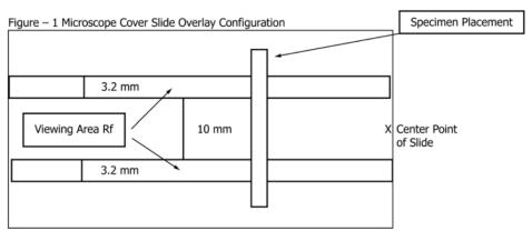
FIG. 1 Microscope Cover Slide Overlay Configuration
